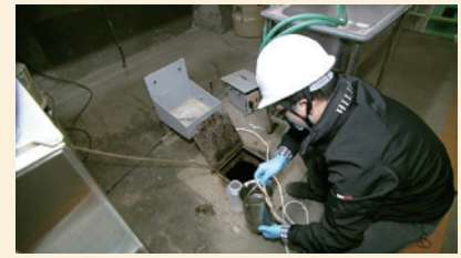
下水処理場でのサンプル収集 Collecting samples at a wastewater treatment plant
